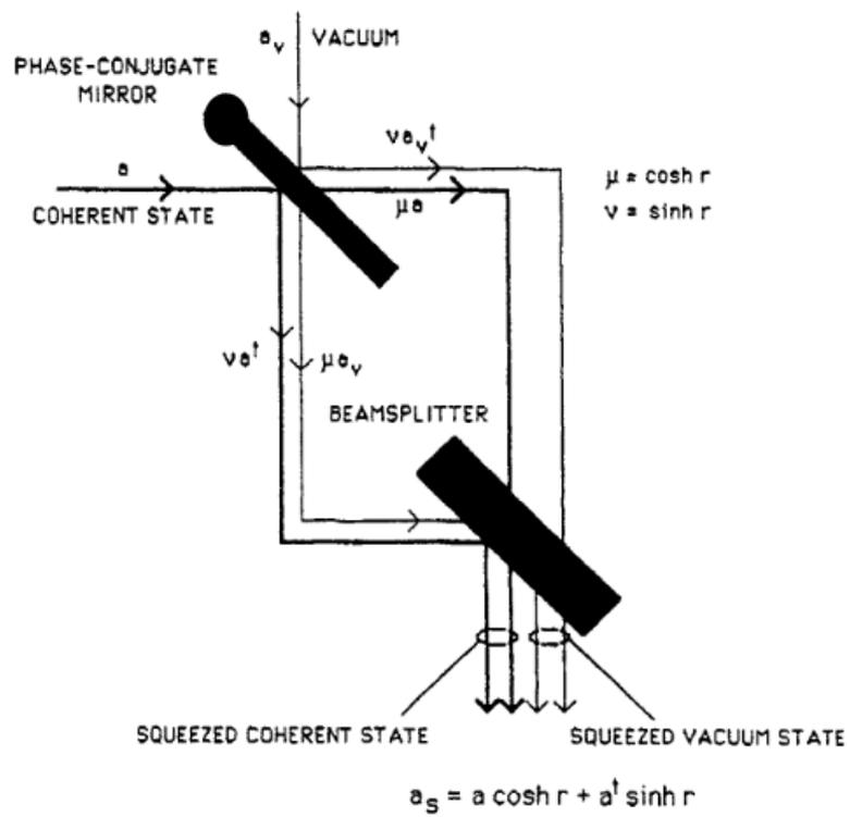
Figure 6.3: Generation of quadrature-squeezed light using a phase-conjugate mirror. [8]
