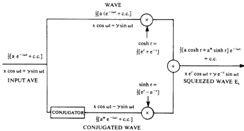
Figure 6.1: Generation of quadrature-squeezed light by the use of a non-linear medium providing phase conjugation)[8]
