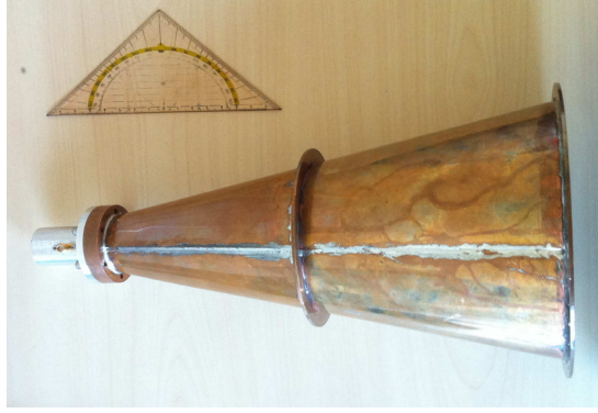
(a) The copper Picket Potter horn with its aluminum waveguide [Lap, 2015].
