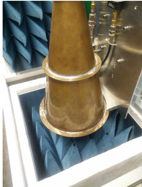
Figure 18: LNB mounted on the horn with its components.
