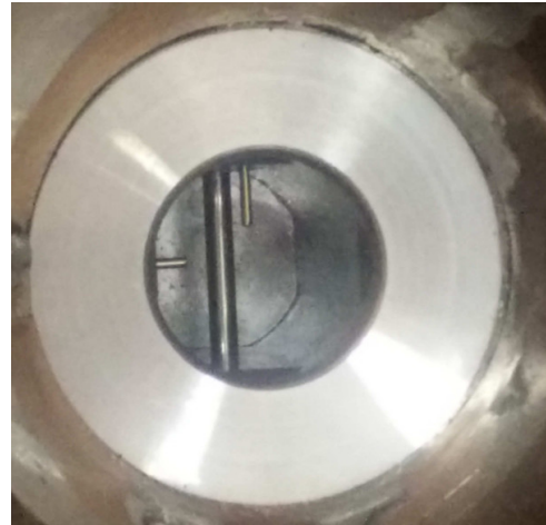
(b) New transition to the LNB (zoomed), clearly the two polarization antennas can be seen. Included is a big pin which serves as filter.
