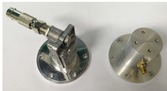
Figure 17: An LNB in the flange compared with the old waveguide.
