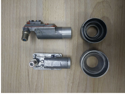
(a) LNBs cut with lathe. Feedhorn is cut off and the outer radius is cut to 20 mm.
