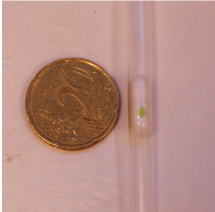
Figure 10: Sample contained within a cotton containing capsule inside a straw, next to a 20ct coin for size comparison. The sample is green because it has reacted with water.
