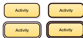
Figure 4.6: Four different states of an activity. The activities on the bottom are mandatory, the activities on the right execution is mandatory.
