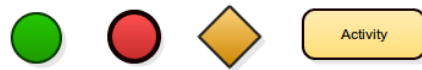
Figure 4.5: Normal BPMN elements which can be used in the editor: a start event, an end event, a gateway and an activity.
