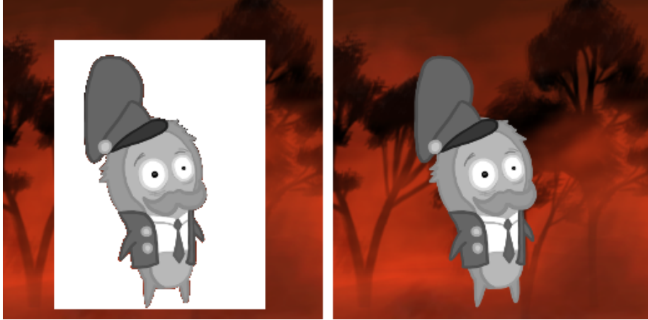
Figure 3.10: A texture in LUMINANCE format (left) and a texture in LUMINANCE_ALPHA format (right).
