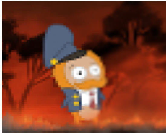
Figure 3.4: Difference between NEAREST (left half) and LINEAR (right half)
