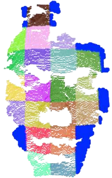
Figure 3.4: The grid (3cm here) is projected orthogonally onto one pose normalized face. Each patch is colored differently, for visualization purposes. The patches colored blue are discarded since the number of pixels in those patches is smaller than the average number of pixels per patch.
