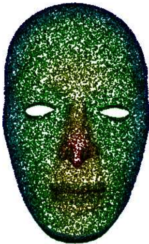
Figure 2.6: Generic 3D face template used for alignment to a common canonical position during ICP.
