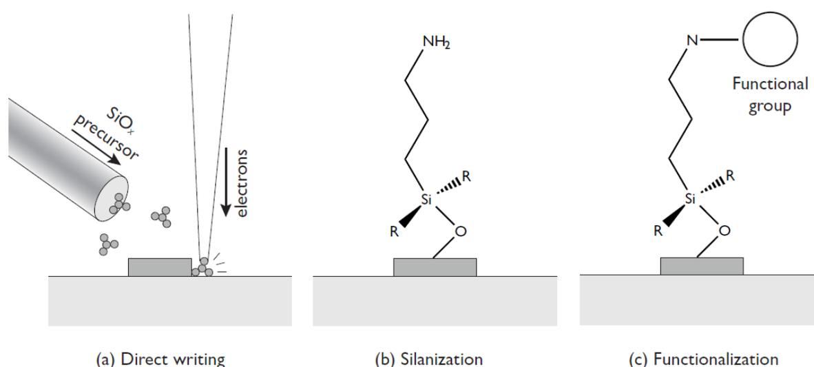
Figure 2.1: The basics of the functionalization process are shown. (a) A silicon oxide gas is exposed to a FEB which creates a deposit on the surface. (b) Silanes from a solution attach to the nanostructures. (c) Functional molecules bind to the silanes. [4]
