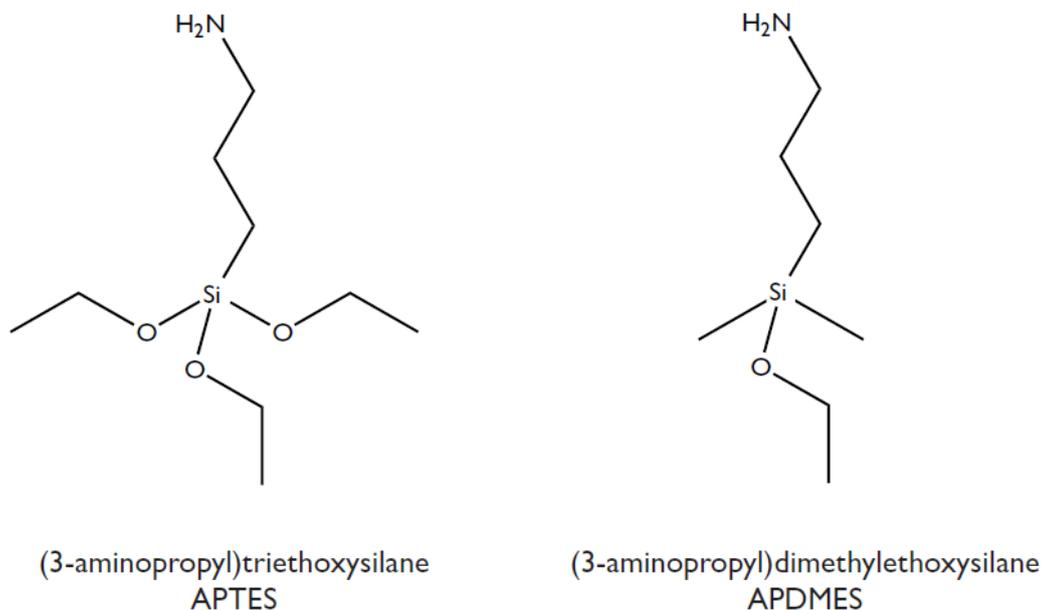
Figure 2.2: The molecular structures of APTES and APDMES.
