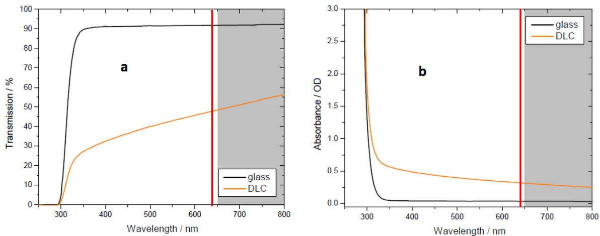
Figure 4.1: (a) Transmission in percentage of incoming light and (b) absorbance properties of DLC coated cover slides. The point of interest is at 637 nm.
