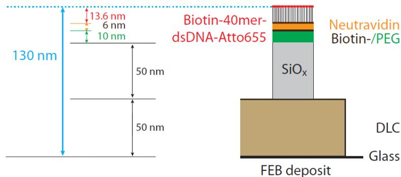
Figure 4.4: An estimation of the height of the FEBID block structures. A stacking of DLC coating (50 nm), silicon oxide (50 nm), PEG (10 nm), neutravidin (6 nm) and dsDNA-ATTO655 (13.6 nm).
