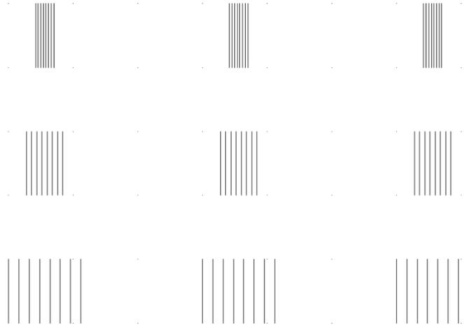
Figure 3.2: The geometry of the line structures. Each set consists of eight lines of 5  $\mu\text{m}$  long. In the third row they're separated by 0.8  $\mu\text{m}$ , in the second row by 0.4  $\mu\text{m}$  and in the first row by 0.2  $\mu\text{m}$ . The accelerating voltage of the field emission gun is 30 keV. In the first column the number of scans is 8k, in the second column it is 16k and in the third column it is 32k. A pitch of 4.5 nm is used.
