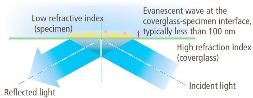
Figure 2.6: An illustration of TIRF [24]. Evanescent waves perpendicular to the surface are generated with an effective range of about 100 nm. The fluorophores in that region will be excited.
