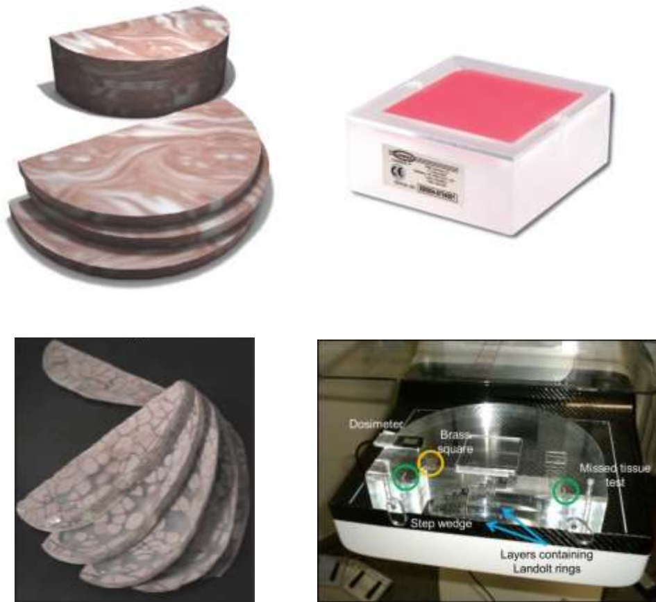
Figure 1. Phantoms investigated by Brunner et al. [12]: a – CIRS BR3D phantom [13]; b – ACR Prototype FFDM Accreditation phantom [14]; c – Penn anthropomorphic phantom [15]; d – Quart mam/digi EPQC phantom [16]
