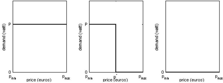
Figure 2.2: typical bid curves for device agents. The left figure shows the bid curve of a device that requires to run, using  $P$  watt. The middle figure shows the curve for a device that has some flexibility and only wishes to run if the price is below  $p^*$ . The right image shows the curve for a device that won't or can't run, thus requiring no power.
