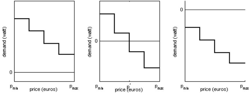
Figure 2.3: Example aggregated bid curves in different balance situations for a PowerMatcher cluster. The right image shows an aggregated bid in a state where there is a deficit of electricity. The middle image shows the aggregated bid in a state where the cluster is balanced. The right image shows the aggregated bid in a state where there is a surplus in the cluster.
