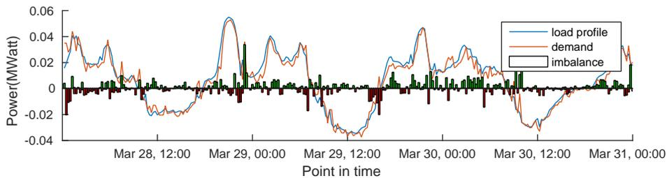
Figure 5.9: Behavior of a cluster using an objective agent that offers all of its available flexibility to the TSO
