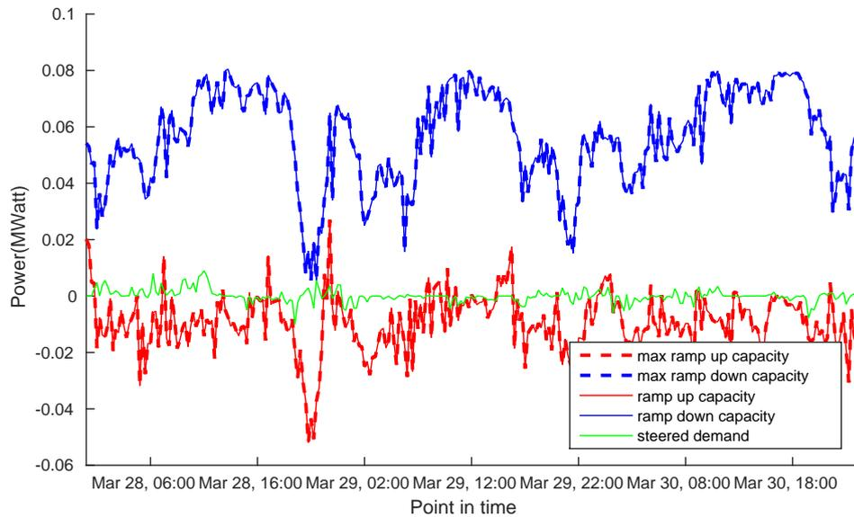
Figure 5.5: Available flexibility, offered flexibility and the adjustment made by the objective agent
