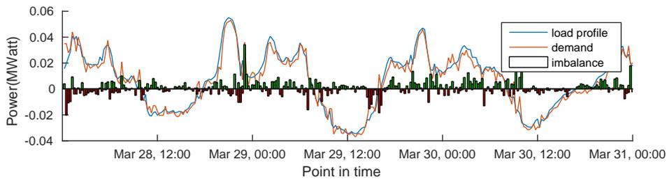
Figure 5.8: Behavior of a cluster using an objective agent that offers 80% of its available flexibility to the TSO
