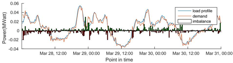
Figure 5.6: Behavior of a cluster using an objective agent that doesn't offer any flexibility to the TSO
