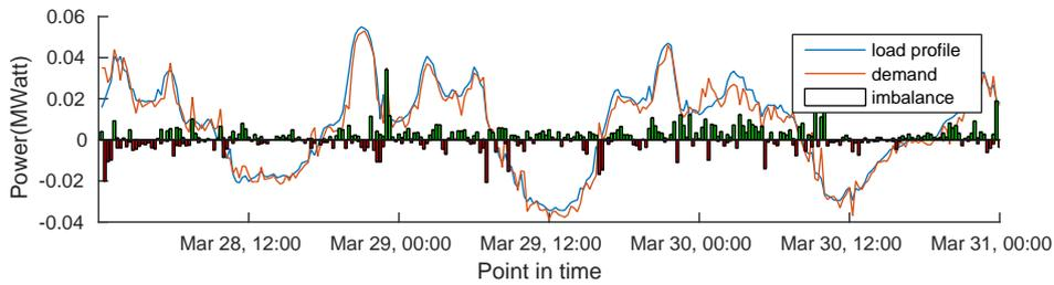
Figure 5.7: Behavior of a cluster using an objective agent that offers 50% of its available flexibility to the TSO
