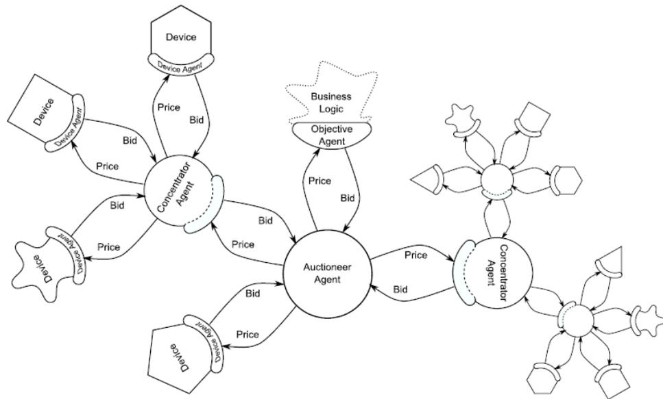
Figure 2.1: A typical PowerMatcher cluster containing each of the four agent types: device agents, concentrator agents, an auctioneer and an objective agent. Adopted from [34]
