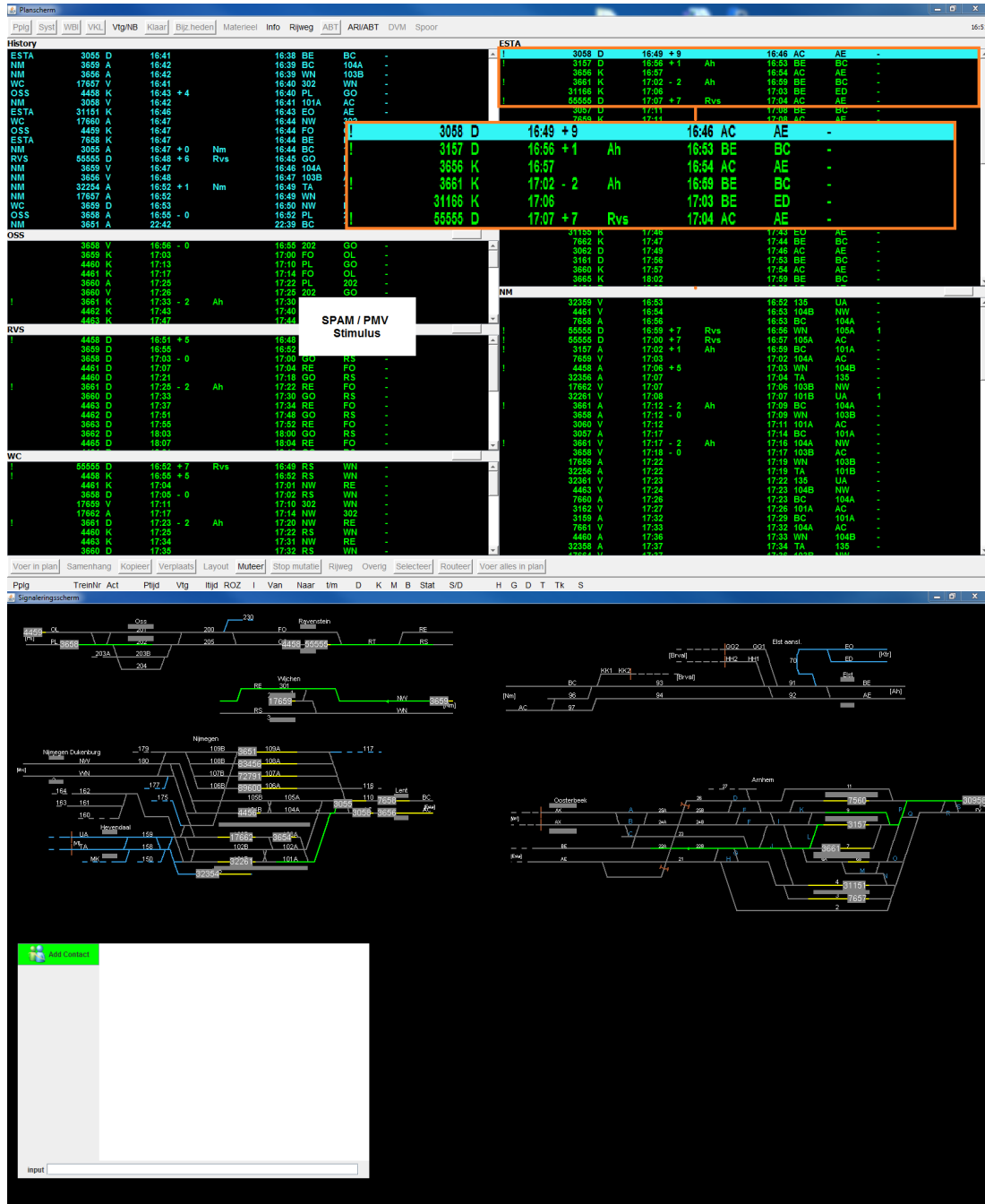
Figure 1: Graphical user interface of the TTC simulator. The top screen is the “planning screen”, with “planning lines” that contain the planned action and time for a train. The white box is the location where the SPAM button and PMV stimuli were depicted. In the bottom “signaling screen” a helicopter view is depicted of the train tracks of the operators responsible area. Moreover, the chat interface was shown on this screen. During the experiment, the two screens were presented side-by-side.
