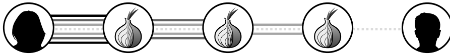
Figure 1.3: Visualisation of onion routing of Alice wrapping her message in layers of encryption and each onion router removing one encryption layer until the message reaches Bob. Source: Spread the word about Tor [73].
