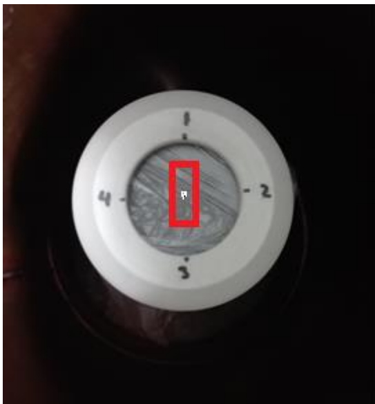
Figure 15 The detector on which the source is placed with numbers relating to the different positions measured
