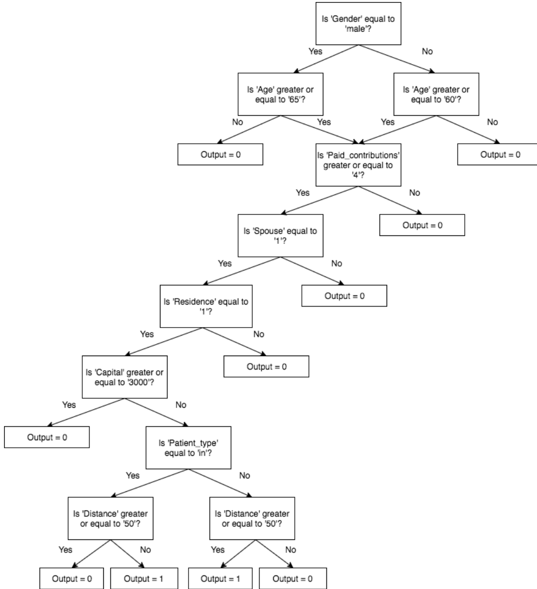
FIGURE 4.1: The expected decision tree that the algorithm will produce, based on the rules that generated the dataset.
