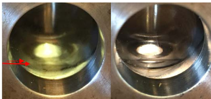
Figure 13 – Results of solubility experiment on n -pentadecane (left) and n -squalane (right) in scCO 2
