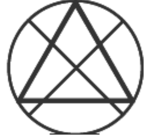
Figure 12: front-view of signal paths through a pipe, each line segment indicates a signal path, thus we see five paths here.
