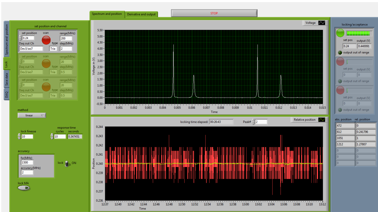
Figure 3.3: The locking program while it is in operation. The top graph shows the signal from the cavity; the two highest peaks correspond to the HeNe laser, while the two smaller peaks correspond to the ECDL. The graph on the lower half of the screen shows the relative position of one of the ECDL peaks over time. The program creates feedback voltages in such a way as to keep this position at the set position, which in this example is 0.24.
