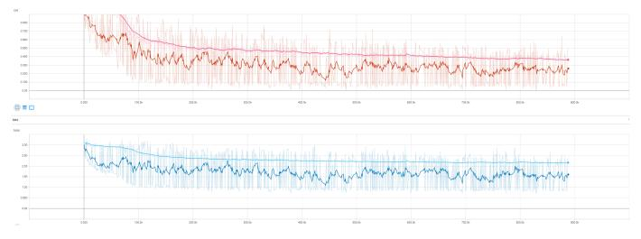
Figure 4.2: CER and Loss of the LAS model on the LibriSpeech100 dataset. Light blue is the validation loss, whereas dark blue describes the train loss. Pink is the validation CER, and red describes the train CER. The x axis is the number of iterations and the y axis is CER/Loss rate.
