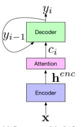
(a) Components of the LAS end-to-end model [16]
