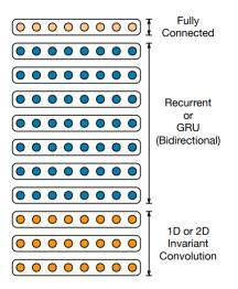
Figure 2.9: Architecture of the DS2 system used to train on both English and Dutch speech [4].
