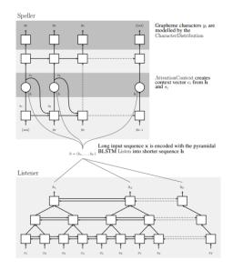
(b) The listener in the LAS model is a pyramidal BLSTM encoding the input x into high level features h, the speller is an attention-based decoder producing the y characters from h [15]
