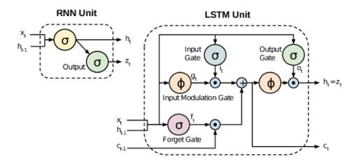
Figure 2.1: Difference between RNN and LSTM units [48].
