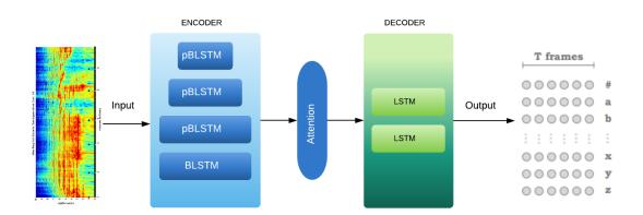
Figure 2.8: The detailed structure of the LAS model's pipeline from input to the output.
