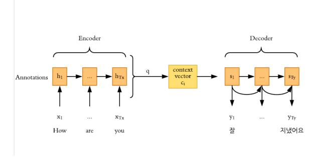
Figure 2.6: An encoder-decoder neural network. An example on machine translation: the input sequence is in English and the output of the system would be in Korean [59].
