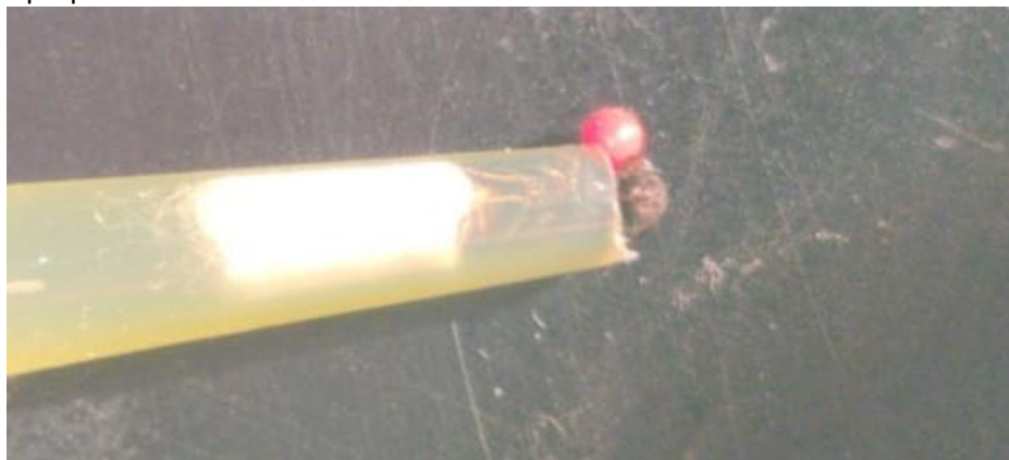
Figure 19. Sample prepared after tube insertion and waxing
