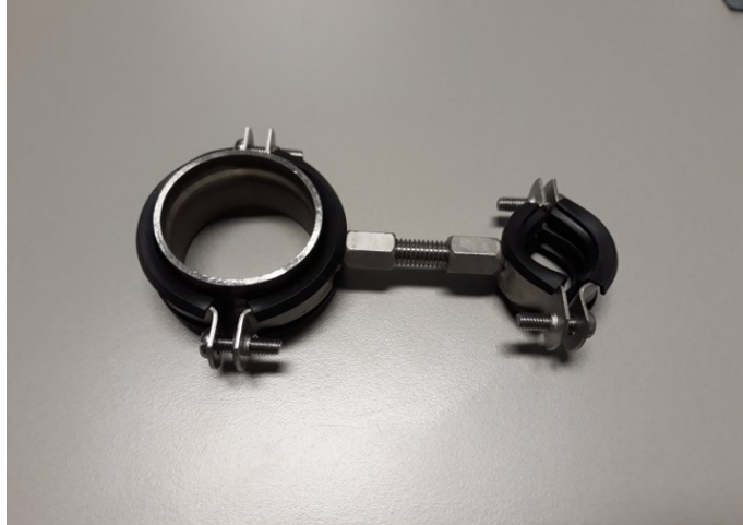
Figure 34: The main pipe is attached to the tower using these pipe clamps. The larger part at the left is clamped to the main pipe and the smaller part at the right side is clamped to the Lutjewad tower.
