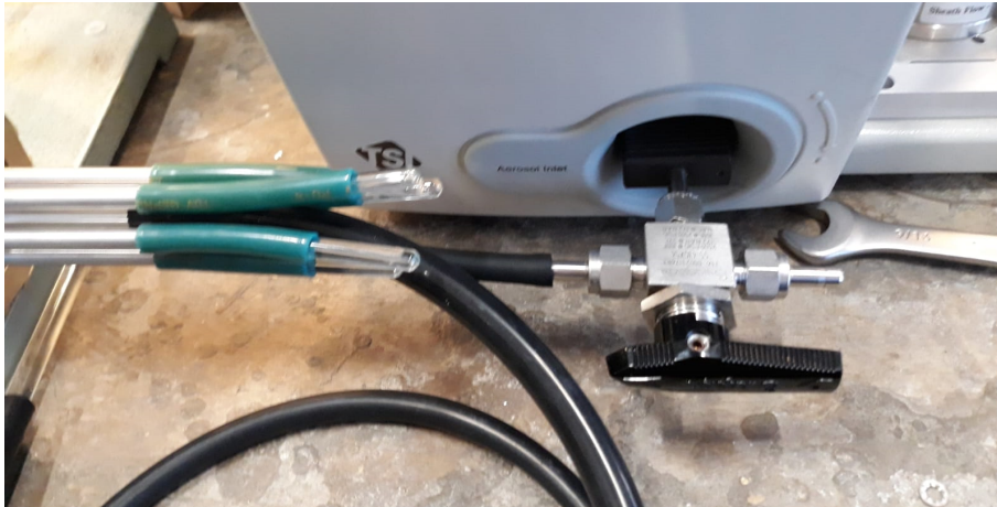
Figure 22: Zoom on the connection from the manifold to the SMPS via the 3-way valve. The valve is now pointed to the setup.
