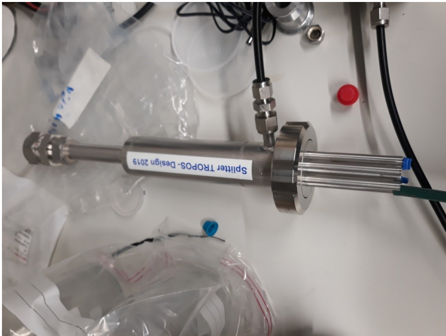
Figure 37: Close up of the manifold. At the left hand side the inlet is seen and at the right hand side the several outlets. The bypass is seen at top top part of the picture.
