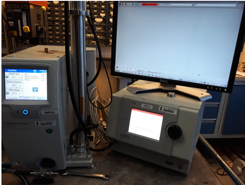
Figure 44: The SMPS used for the calibration. Left is the DMA column seen and at the right side the CPC is seen. The SMPS that will be placed in the container at Lutjewad will be different.
