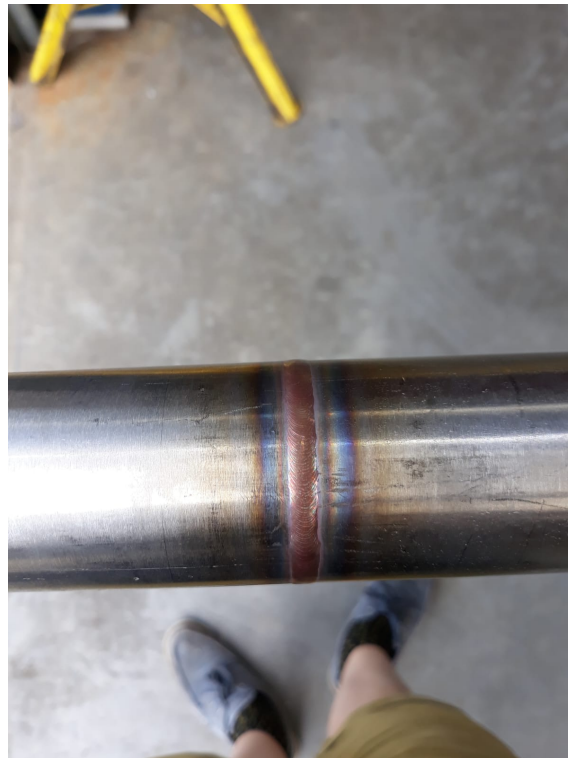
Figure 32: Close up of orbital weld on the main pipe.
