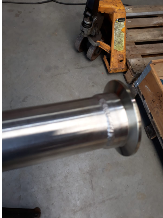
Figure 33: Lower end of the main pipe with the DN50 flange.
