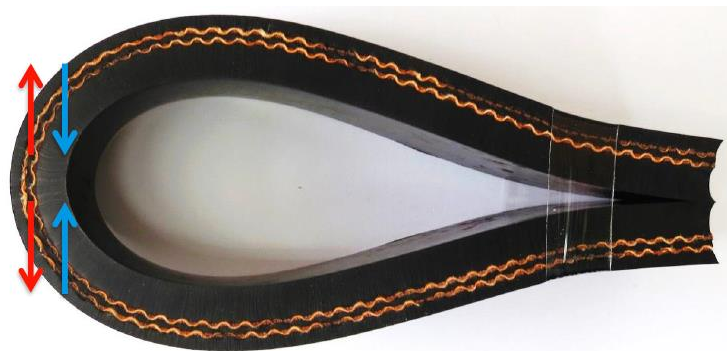
Figure 2. 11: Bending characteristics of rubber membranes. Retrieved from (Gurt, 2015)
