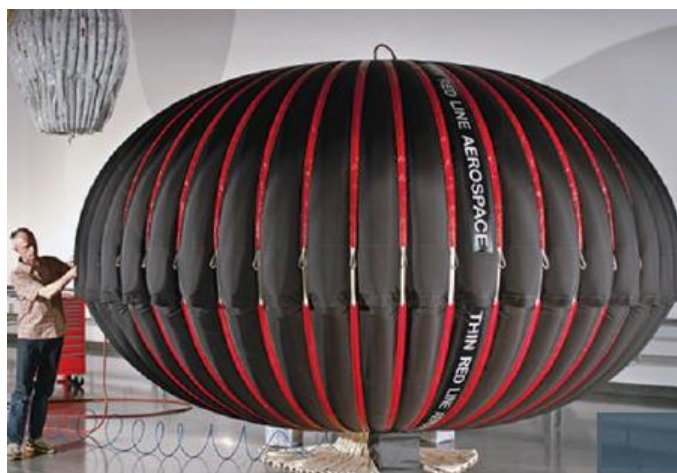
Figure 2. 1: Ultra High Performance Vessel (Thin Red Line Aerospace). Retrieved from M. Pagitz et al. (2007).
