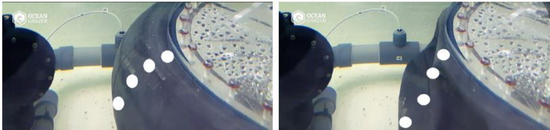
Figure 2. 6: Left: Fully inflated bladder, right: Fully deflated bladder when the folds was formed. Retrieved from (Ocean Grazer, 2015)
