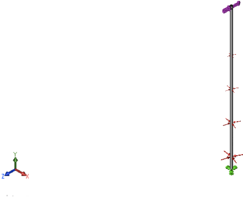
Figure 29: Isometric view of loads and fixtures applied on the umbilical in Solidworks
