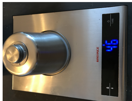
(b) Weight of stainless steel part (46 gr)
