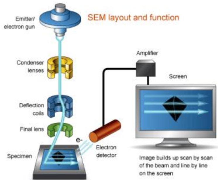
Fig. 4.1: Overview of the Scanning Electron Microscope Technique (SEM) used for analyzing the microstructure of a material [27]
