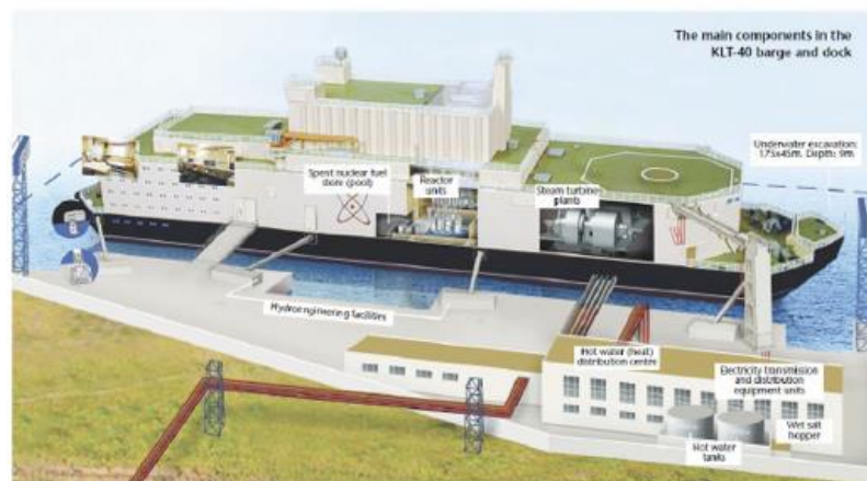
Figure 4: Barge-mounted KTL-40 reactor [6].
