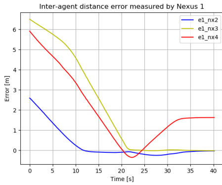
(c) The inter-agent distance error measurement of Nexus 1 during the second try of position 2 in zone 3 for formation 2 ( a = 5, b = 5 )
