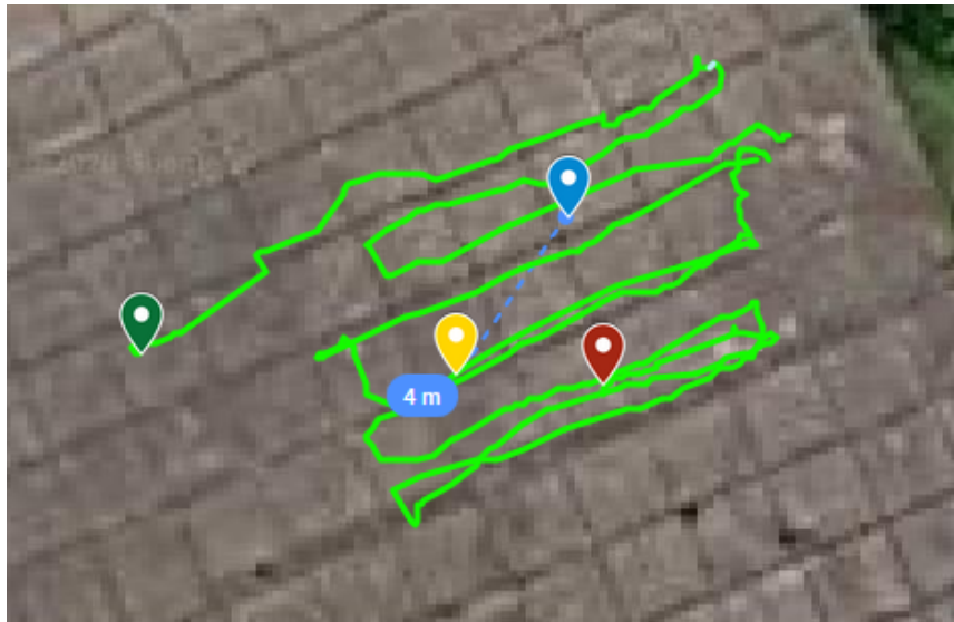
Figure 28: The path of flight 2 shown on top of a satellite image. The green marker indicates the starting point, the red marker indicates the end the blue marker indicates the source location and the yellow marker indicates the location with the highest measured count rate.
