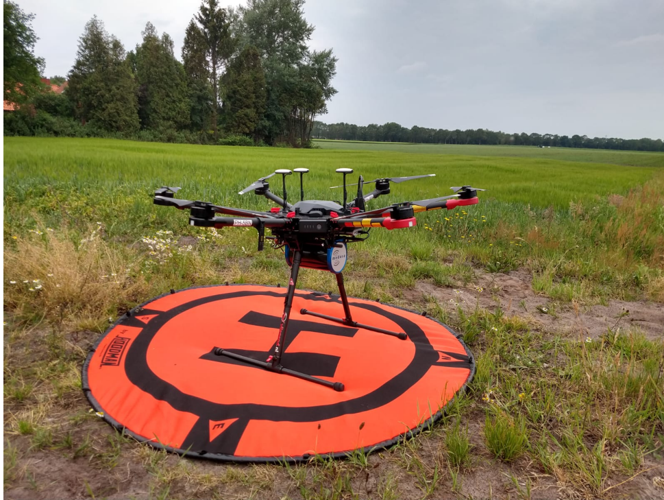
Figure 19: The DJI Matrice 600 pro setup with the MS350 mounted underneath it.
