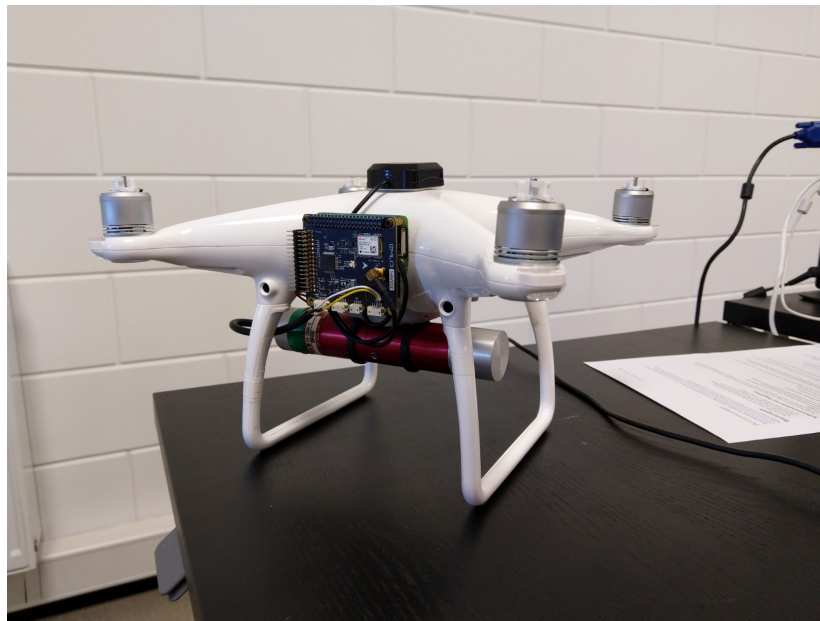
Figure 18: The customized DJI phantom 4 with the 12.8 ml CeBr 3 crystal detector.
