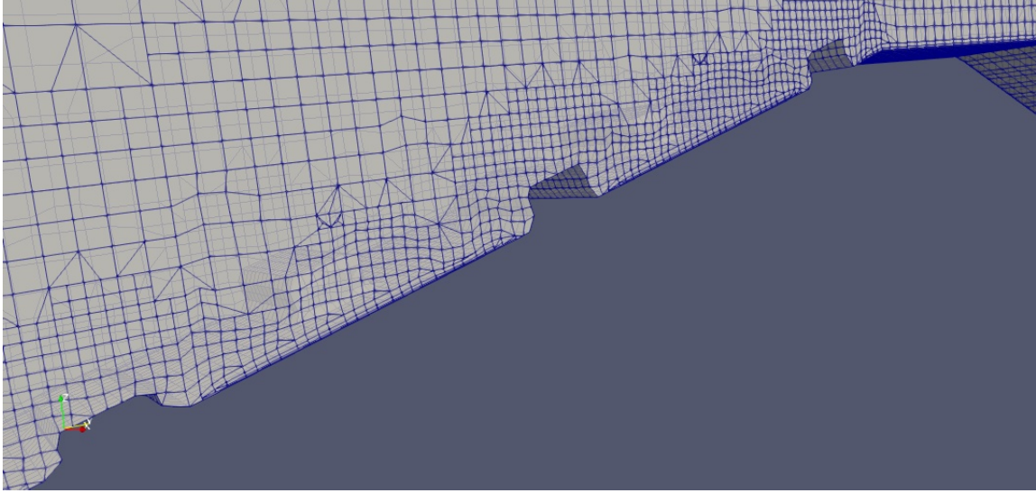
Figure 11.2: A cross-section of the mesh of the upper slope with the ribs.
