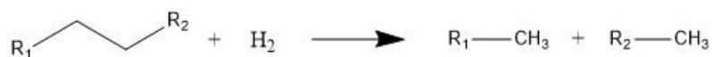
Figure 16: Showing a possible hydrocracking reaction, which requires the presence of a catalyst [48].
