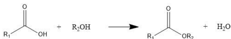
Figure 17: Showing a possible esterification reaction, where a carboxylic acid is converted to an ester along with the formation of water [48].
