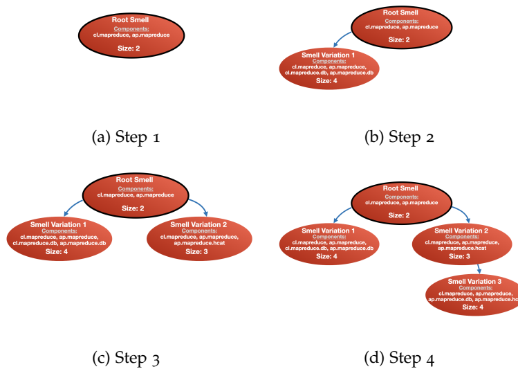
Figure 13: Step 1 to 4 of creating smell tree 24 of Sqoop. There is one splitting at the root which is indicated by a black frame.
