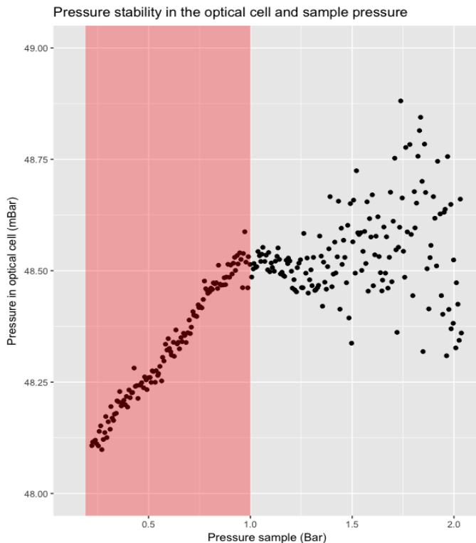
Figure 4, pressure stability in the optical cell of the SICAS and sample pressure. This chart shows the results of pressure in the optical cell versus the sample pressure. Moreover, this chart shows that the pressure of the sample has to be around 1 bar to have a stable pressure in the optical cell. Finally, the red highlighted range of the chart shows the most stable pressure of the optical cell.
