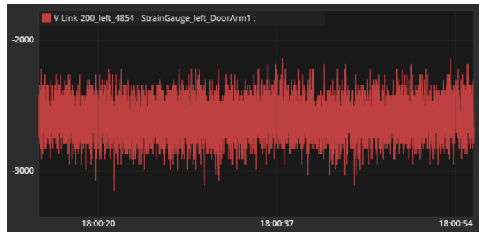
Figure 3.3: Noise dominated signal from the upper door arms strain gauge.
