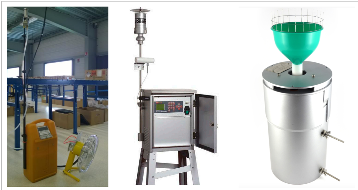
Figure 6: From left to right, Deltanova GH300 Air Sampler ( Dris et al., 2017 ), TECORA, ECHO PM Sampler ( Abbassi et al., 2018 ) and Palmex Rain Sampler ( Allen et al., 2019 ).
