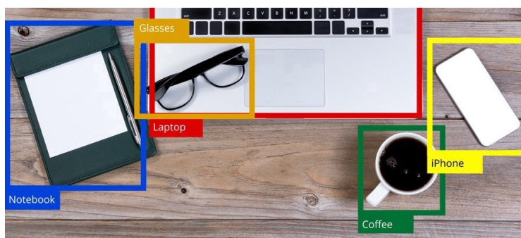
Figure 2.1.: Illustration of bounding boxes around objects in an image
