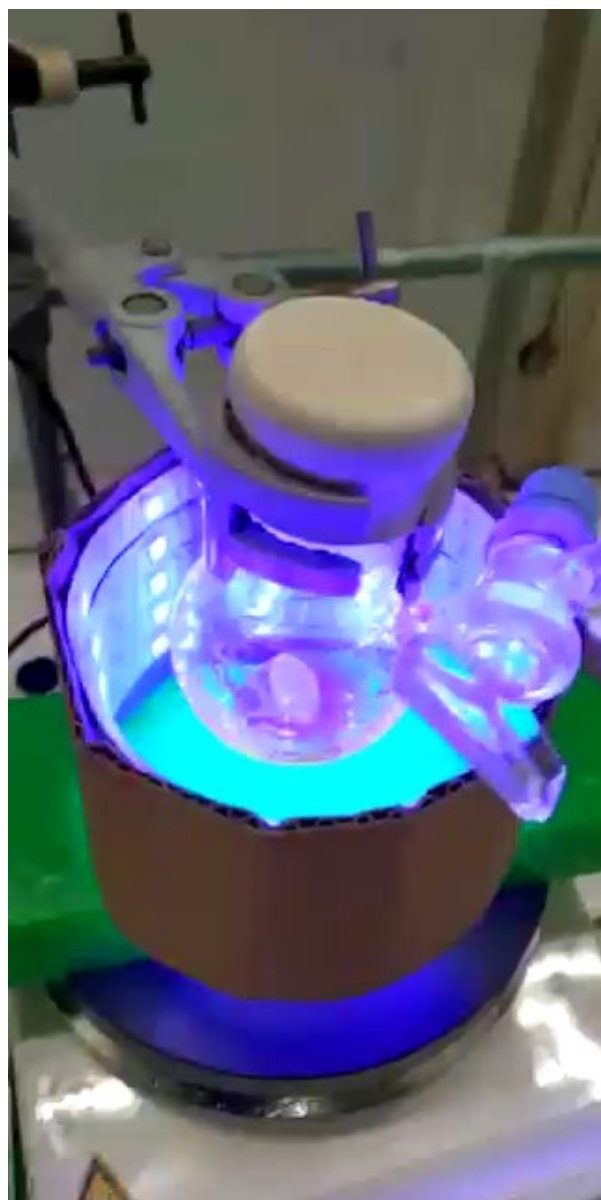
Figure 13 A close up photograph of the reaction setup for the photocatalytic removal of the CTA.
