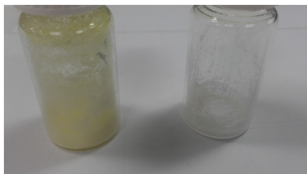
Figure 15 The two different polystyrene polymers. On the left is the regular PS with CTA and on the right the new PS without CTA.
