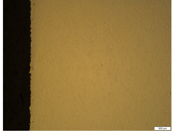
Figure 35: Polished microstructure of sample E5, printed at 18 m/s. Magnification factor is 2.5x.
