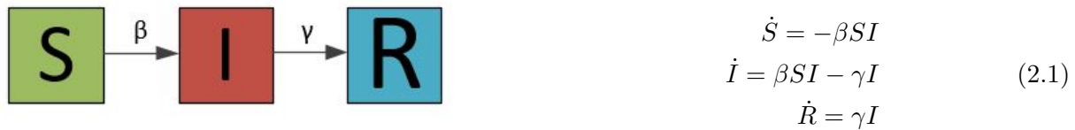
Figure 2.1: Schematic representation of the SIR model. Showing the compartments and its interrelations on the left and the corresponding differential equations on the right
