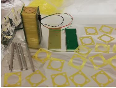
Figure 3.6: Ion funnel with two side plates, rods and the insulating spacer plates removed.
