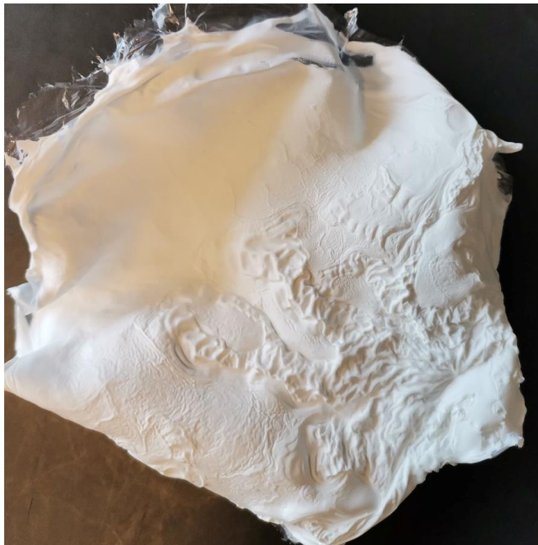
Figure 31 - Film obtained via solvent casting of PLA with acetone as solvent
