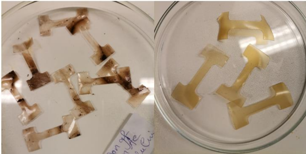
Figure 35 - Cut samples: non-acetylated, non-grafted lignin-PLA blend (left) vs. non-acetylated grafted lignin-PLA blend (right)
