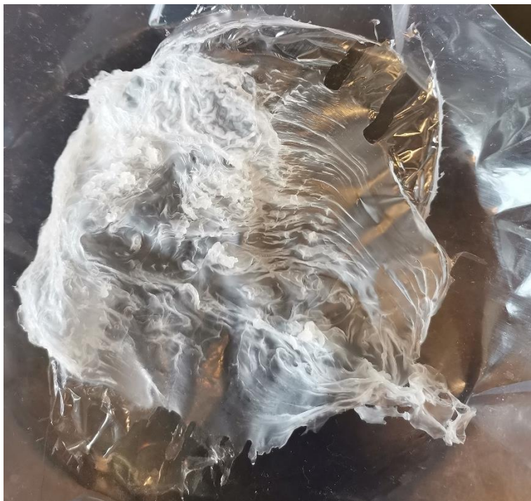
Figure 33 - Film obtained via solvent casting of PLA with dimethyl carbonate (DMC) as solvent
