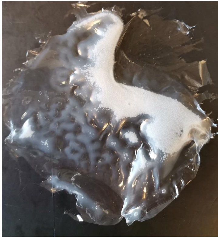
Figure 32 - Film obtained via solvent casting of PLA with p-dioxane as solvent
