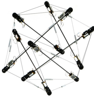
Figure 1: Example of a tensegrity robot consisting of cables and rods (Fivat S. et al 2010)
