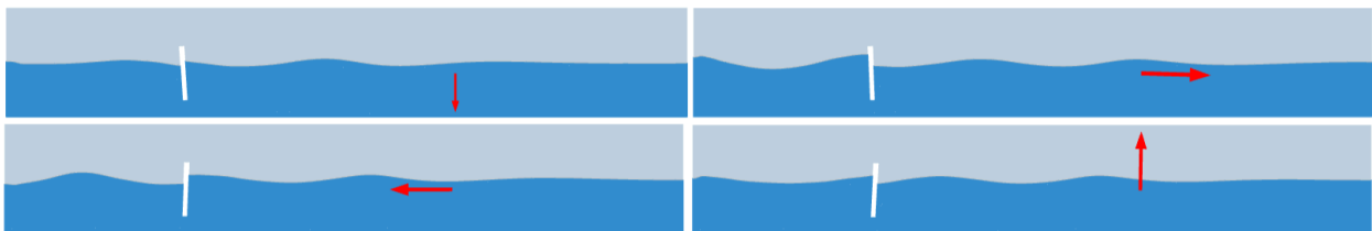
Figure 39: Particle motion using flap type wavemaker, scaled arrow.
