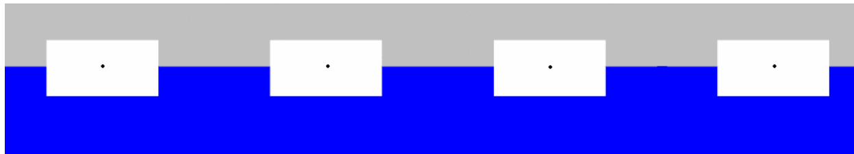
Figure 64: Example for case 1 where the black dots represent the center of mass, connection to the PTO and most importantly the fixed point, to fix the floaters in surge.
