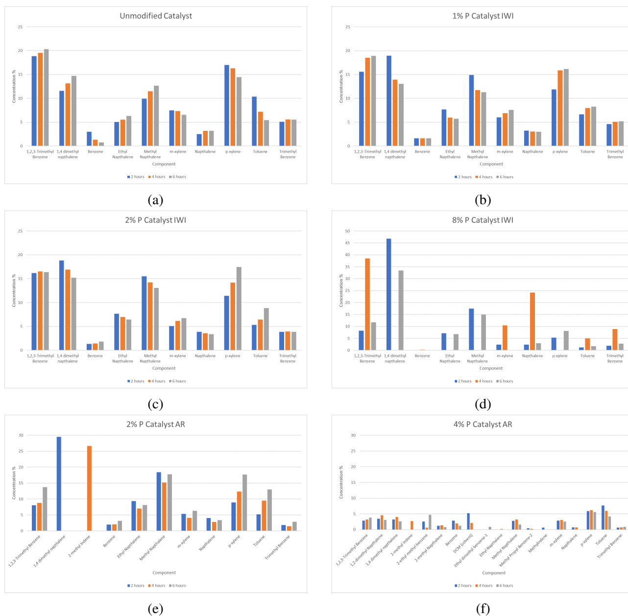
Figure 15: Detailed depiction of liquid products in samples taken after 2, 4 and 6 hours for unmodified ZSM-5 catalyst (a), 1% IWI catalyst (b), 2% IWI catalyst (c), 8% IWI catalyst (d), 2% AR catalyst (e) and 4% AR catalyst (f)
