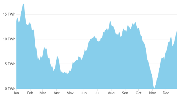
Figure 5 - Example of ETM graph displaying total energetic value of hydrogen stored throughout the year
