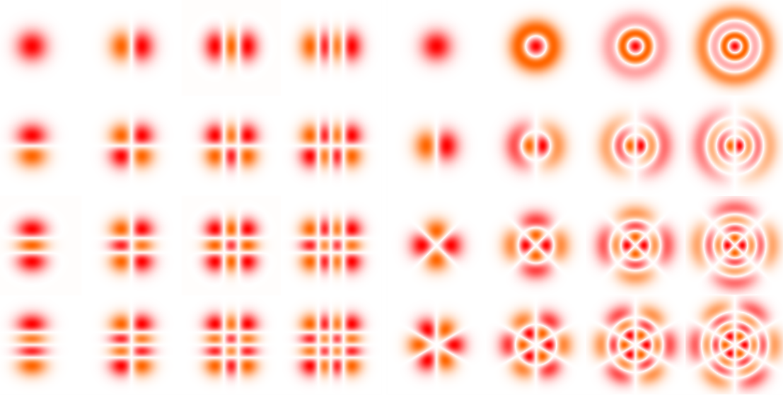
Figure 2: Hermite-Gaussian modes, starting from TEM_{00} , m increases from left to right, n increases from top to bottom. Plotted is the the real part of the electric field. Red indicates a positive value for the field, orange negative. [Self, A.1]
