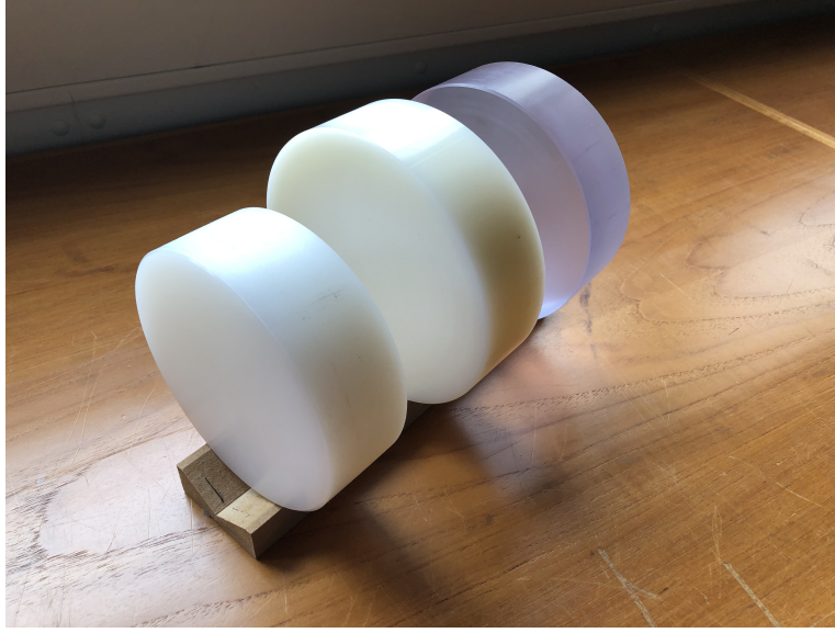
Figure 8: The three samples of polyethylene (PE), polycarbonate (PC) and nylon. Each had a thickness of 4 cm.
