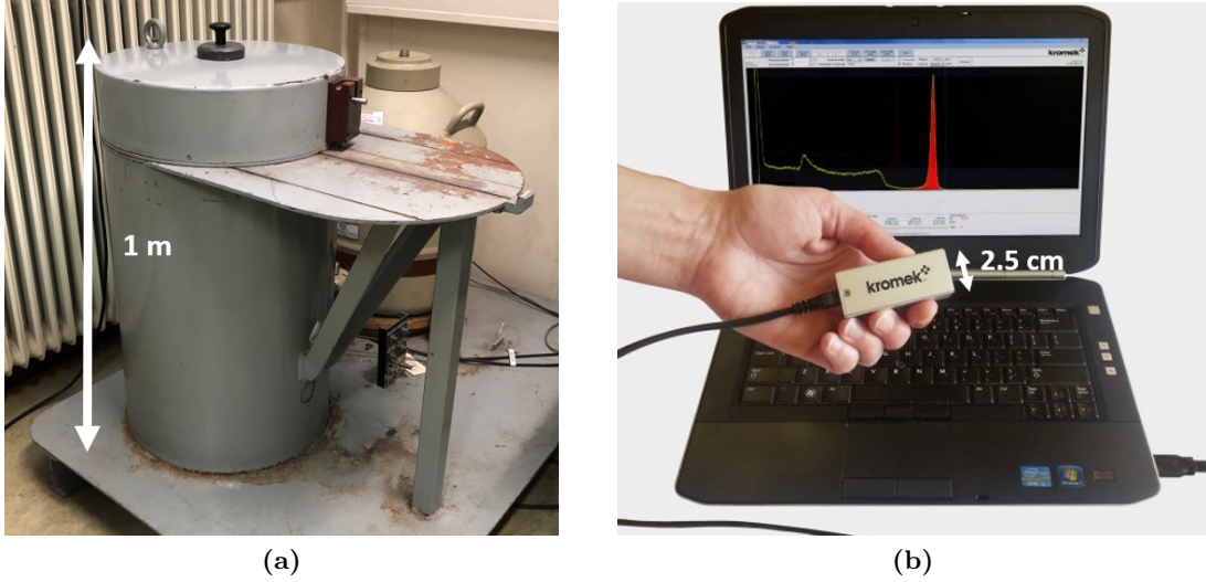
Figure 4: (a) The HPGe detector with a height of roughly 1 m. (b) The Kromek GR1 CZT detector with a width of 2.5 cm[21].
