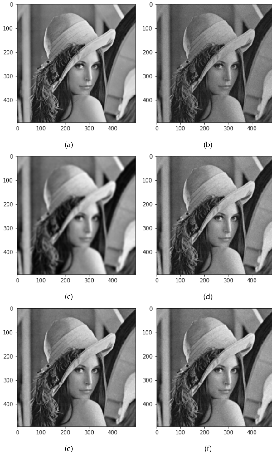
Figure 3.9: Overview of the original and the smoothed images of Lena, where the following images are presented: (a) Gray-scale Lena, (b) Lena with Noise, (c) Gaussian Blur with \sigma = 3 , (d) Optimal Gaussian Blur, (e) Optimal Perona-Malik Diffusion, (f) Optimal KDEsmoother.
