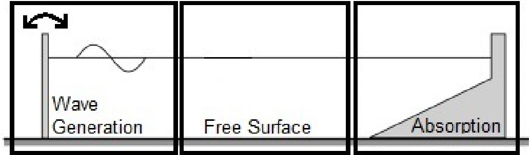
Figure 12: Schematic of a generic wavetank including the wave generation, free surface and absorption zones [13].
