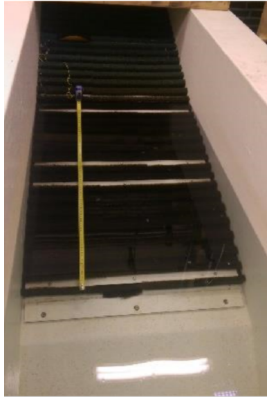
Figure 15: The foam layer installed at the beach in the wave tank.
