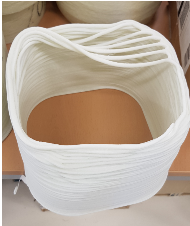
Figure 1.2: Small layer-time results in a collapse
