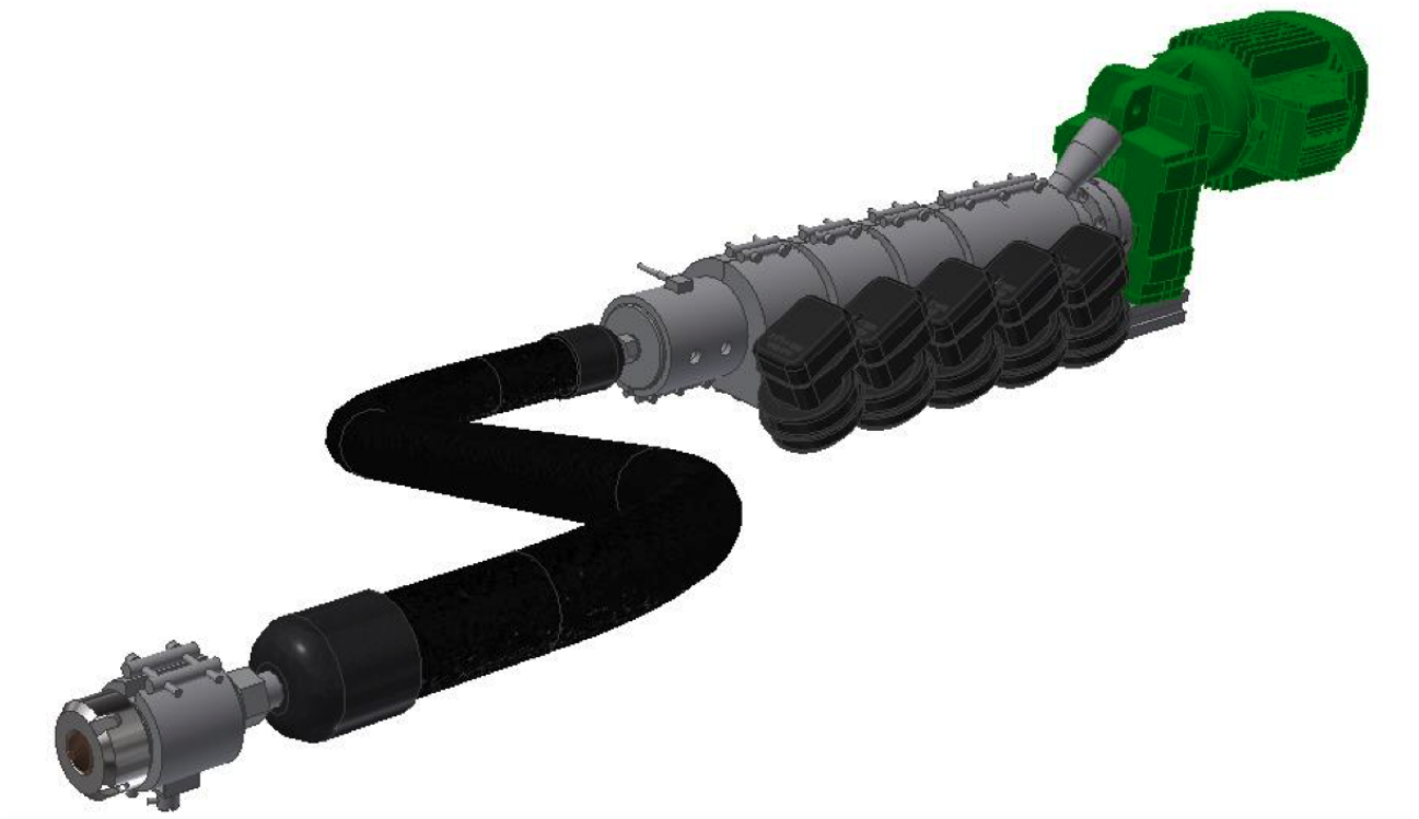
Figure 1.5: 3D CAD model of the Xtrution granulate extruder
