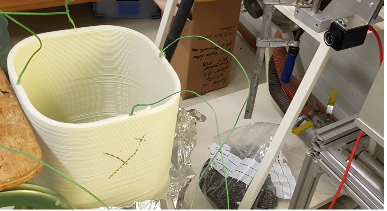
Figure 4.9: Experiment set-up for determining the emissivity of the material
