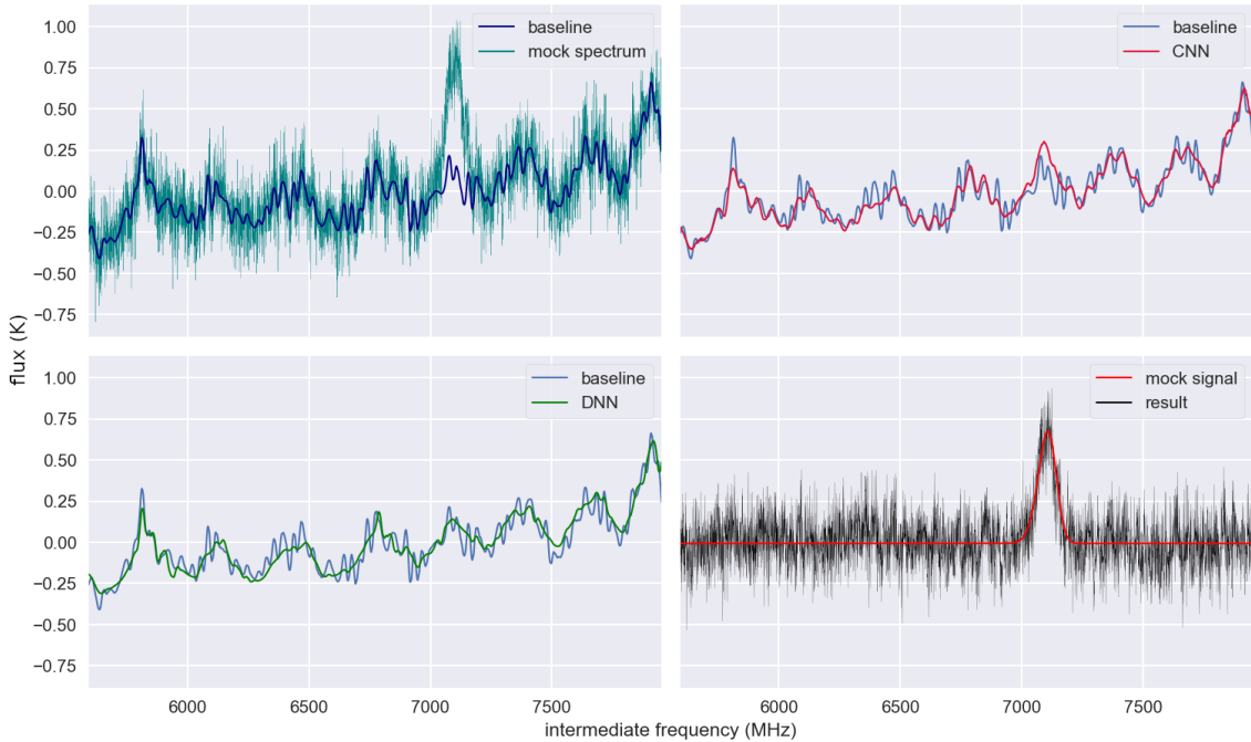
Figure 8.2: Intermediate results on a mock spectrum, at each step in the algorithm. The top left panel shows the mock spectrum, and the corresponding smoothed stability spectrum that was used for the baseline. The top right panel compares the baseline with the result of the CNN, after it is applied to the mock spectrum. The bottom left panel compares the baseline to the result of the PCA and dense neural network. The bottom right panel gives the original mock signal, compared to the baseline corrected mock spectrum. For easy comparison, in this figure, all spectra have the same data shape and are scaled to the physical amplitude in Kelvin.
