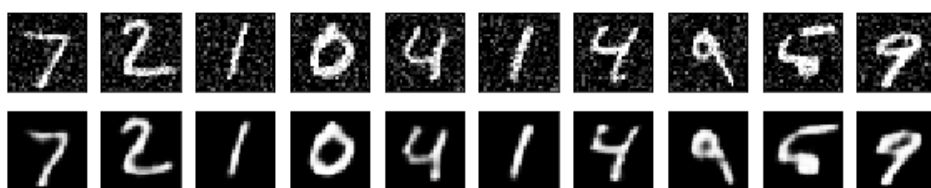
Figure 5.7: Autoencoders can be used for noise reduction. In this case, an autoencoder was trained to reproduce images of handwritten numbers from the MNIST dataset. After a sufficient amount of training, the network is able to reproduce the numbers. If the network is then fed noisy images (shown in the top row), it will output relatively noiseless images (bottom row).
