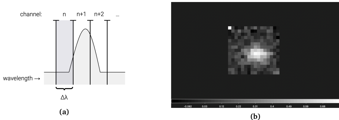
Figure 2.2: a) Diagram showing how a spectral pixel (channel) represents a window of certain width \Delta\lambda in the total spectrum obtained in one spatial pixel. b) Channel in the data cube of a galaxy from the KMOS 3D survey (GS4_12401) showing clear H \alpha emission. SAOImageDS9 (Joye and Mandel, 2003) is used to display the data cube. Units of the cube are \text{W m}^2 \mu\text{m}^{-1} .
