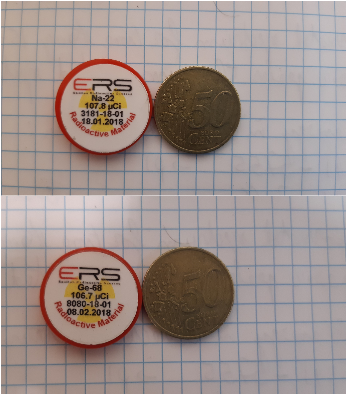
Figure 4.6: ^{22}\text{Na} -source and ^{68}\text{Ge} -source used for this thesis with coin for scale.
