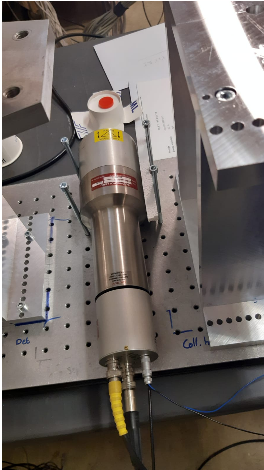
Figure 6.2: The NaI-detector whose PMT can be pulsed by being connected to a pulsed voltage source. This NaI-detector will replace the NaI-detector used in this thesis in future sessions.
